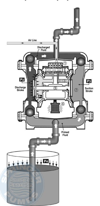
Air-Operated Double Diaphragm (AODD) pumps are powered by compressed air or nitrogen.
